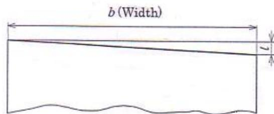
**Figure 1 Out-of-square for flat sheet**
