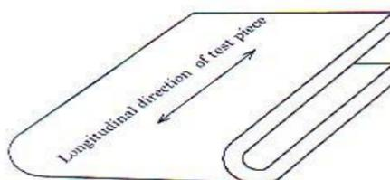
**Figure 2 Direction of bend test**
