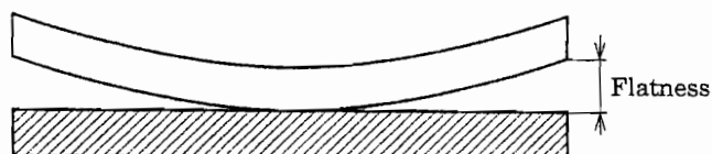
Figure 2 Measurement of flatness
